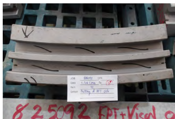
Fig.24 Heavy frettage on FWD side-Body.
