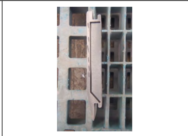
Fig.14 Severe degradation on tip shoe (inner plate).
