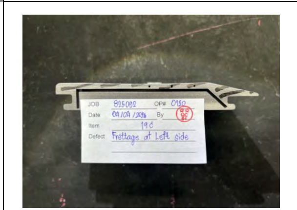
Fig.28 Heavy fretting on left side-Tip shoe.
