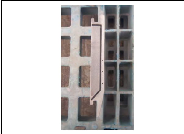
Fig.13 Severe degradation on tip shoe (inner plate).
