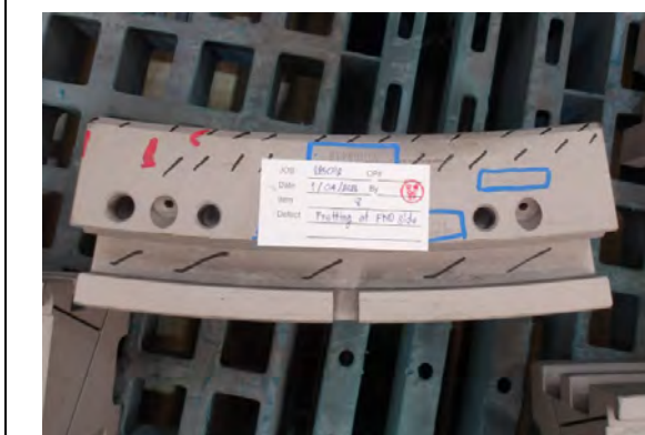
Fig.23 Heavy frettage on FWD side-Body.
