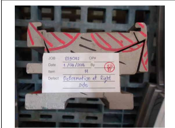
Fig.15 Heavy deformation on right side-Body.
