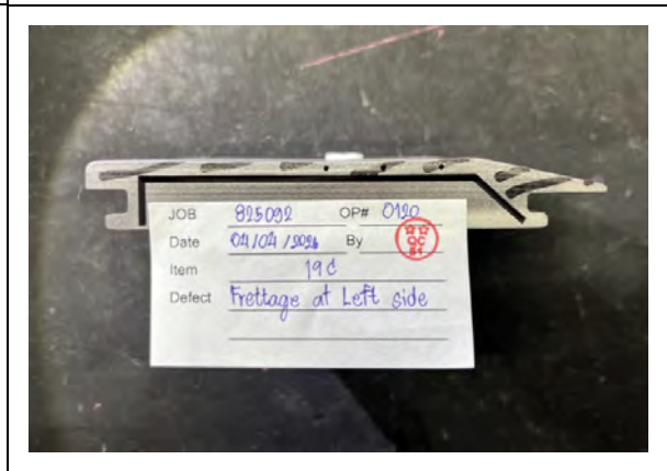
Fig.30 Heavy fretting on left side-Tip shoe.
