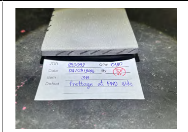
Fig.26 Heavy fretting on FWD side-Tip shoe.
