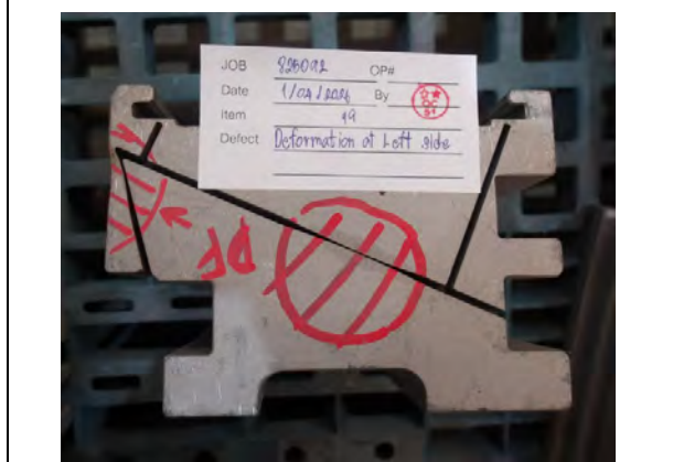
Fig.18 Heavy deformation on left side-Body.
