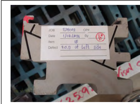
Fig.19 Heavy FOD damaged on left side-Body.
