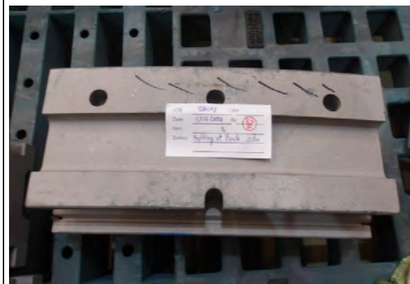
Fig.21 Heavy frettage on back side - Body.
