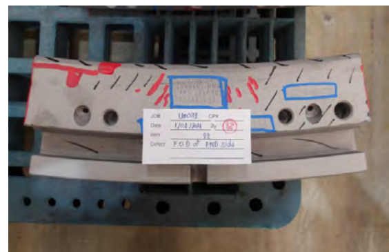
Fig.22 Heavy FOD damage on FWD side-Body.
