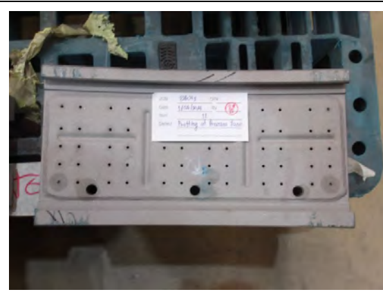
Fig.20 Heavy frettage on pressure face-Body.
