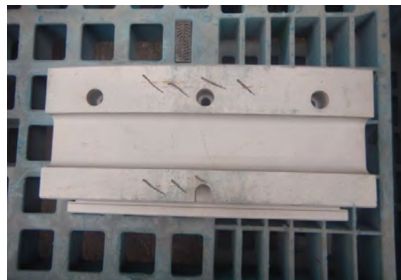
Fig.6 Tear & Wear shroud block body
