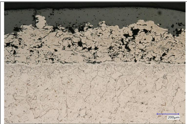
Fig.1 Heavy coating degradation exposing base metal
