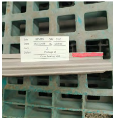
Fig.23 Fretting on outer floating seal.
