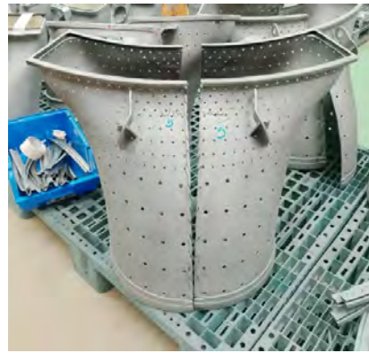
Fig.8 Typical condition of impingement sleeve.
