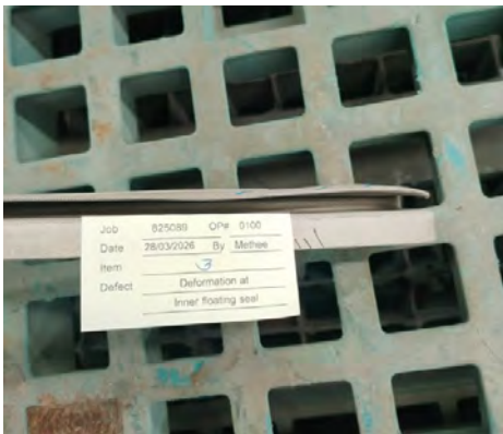
Fig.21 Deformation on inner floating seal.
