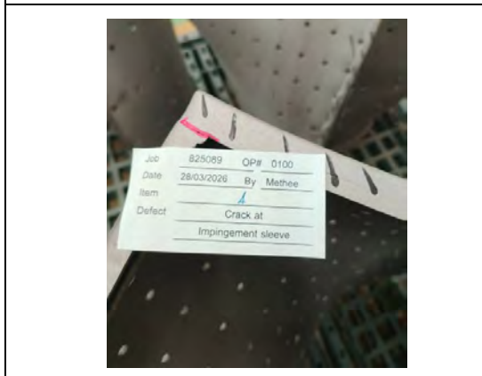
Fig.27 Crack on impingement sleeve.
