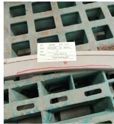
Fig.24 Deformation on outer floating seal.
