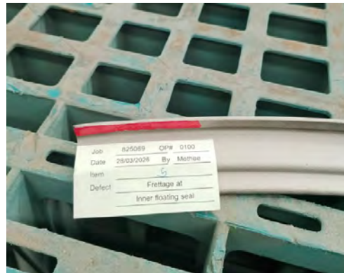
Fig.22 Fretting on inner floating seal.
