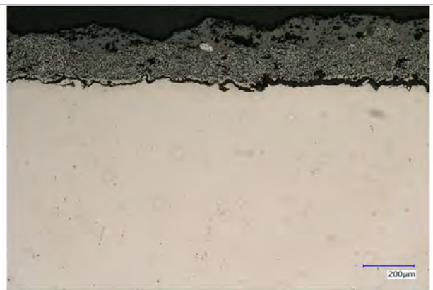
Fig.1 Showing the hot gas path coating and substrate condition.(Etched)
