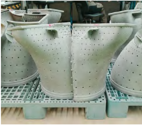
Fig.9 Typical condition of impingement sleeve.
