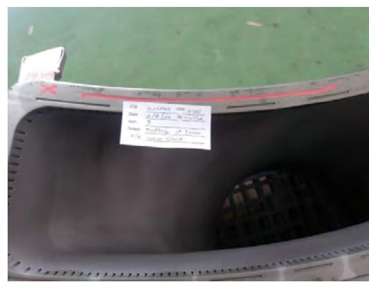
Fig.12 Frettage on inner picture frame wear strip.
