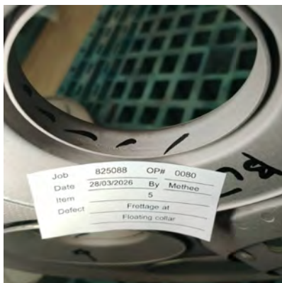
Fig.23 Frettage on floating collar.
