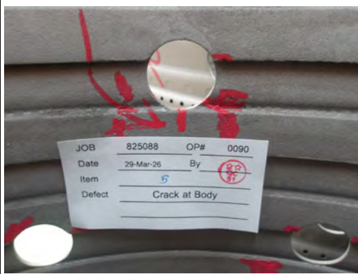
Fig.17 Crack across entire body.
