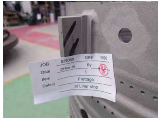
Fig.20 Heavy frettage on liner stop.
