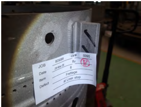
Fig.21 Heavy frettage on liner stop.
