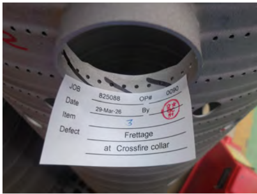
Fig.19 Heavyfrettage on crossfire collar.
