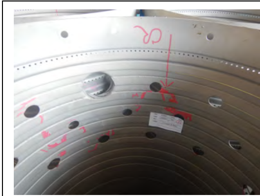
Fig.13 Several heavy corrosion on internal body.
