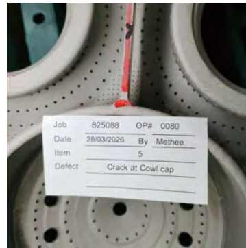
Fig.22 Heavy crack on cowl cap.
