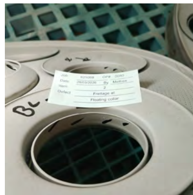
Fig.24 Frettage on floating collar.
