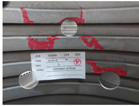
Fig.16 Heavy corrosion across body.
